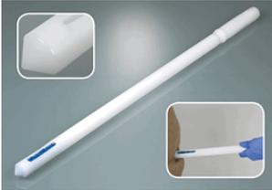
**Description** TargetDispo is used to take a target point sample at a position in the sample material that has previously been precisely determined. The sampler pierces into the powder or granulate while closed. When it reaches the sample removal point it is opened and then closed again. In this way a precise target-point sample is obtained. The sample can simply be emptied through the open handle.
